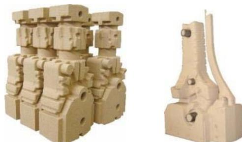
In addition, at Z84200 machines with Vacuum core technology are produced other large cores, such as large engine block cores and hooks.
