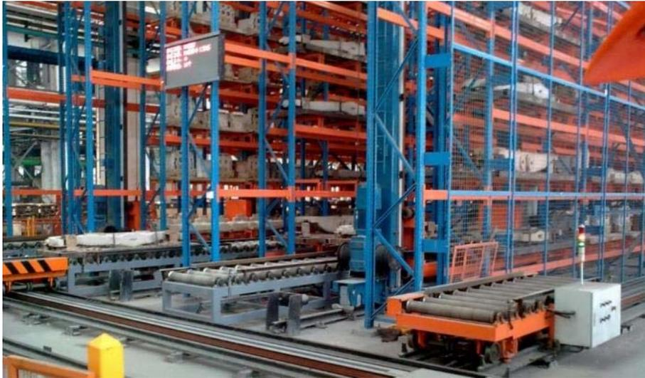
**Automatic handling system for central cores for Railway castings bolster and frame, including**
