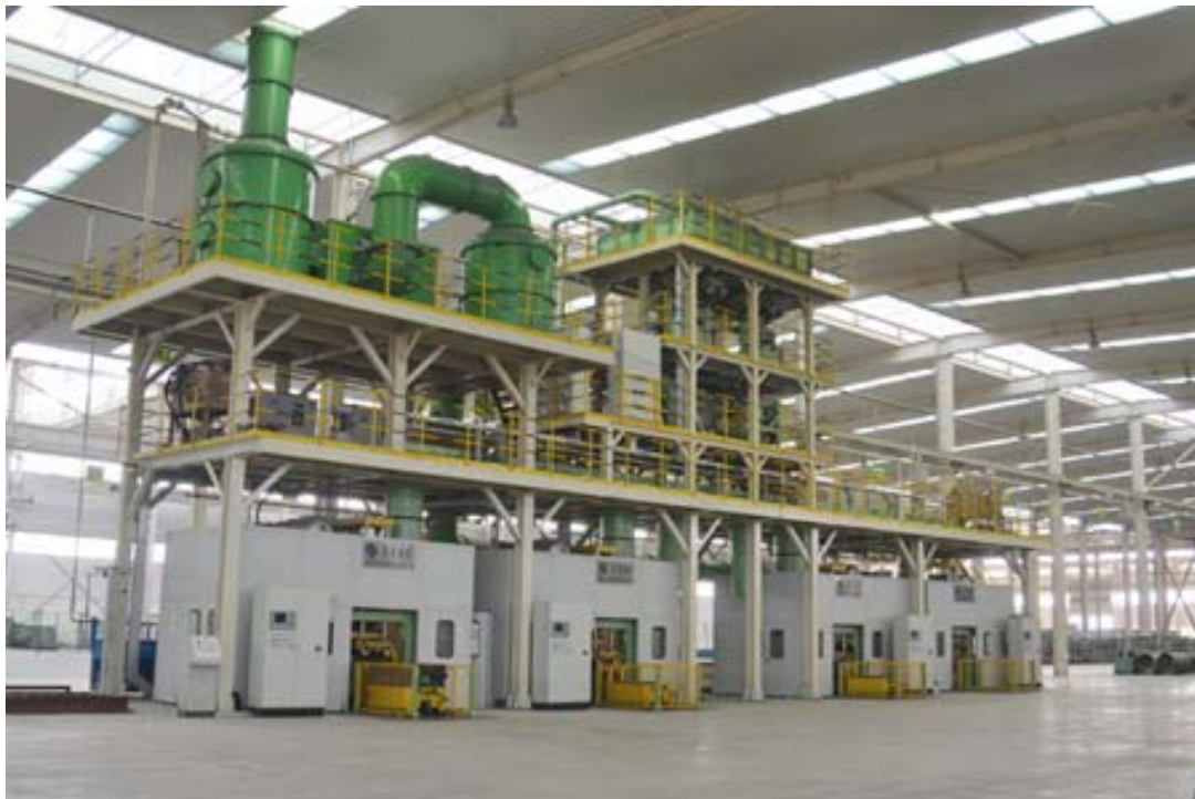
Core machines Z84 series with central sand mixer and sand supply
